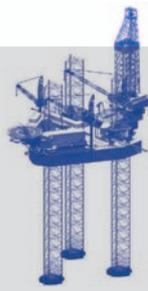
**meters:** That is the length of the three legs supporting the ENSCO 121 drilling platform. It is one of the most modern offshore rigs worldwide. It will be deployed by Wintershall Noordzee in the southern North Sea for up to twelve wells.
